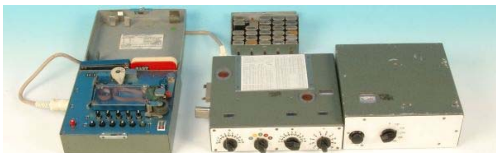
Illustration 13 Old SW transmitter with burst encoder (scanning of a punched tape)
