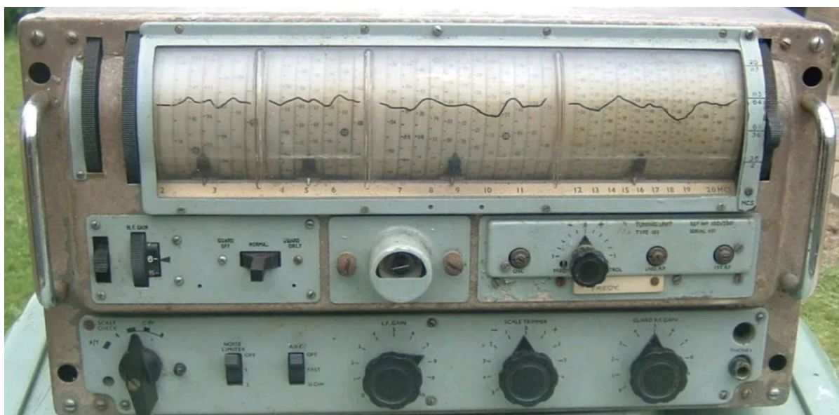
Radio receiver used in RAF intercept stations set rooms, sometimes one atop another; Marconi 1475 [credit unknown]
